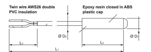
D1 = 9mm D2 = 4mm L1 = 1250mm L2 = 49mm
